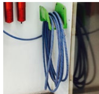
Heated hose system. Independent of ambient temperature.
