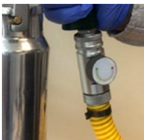
Product regulator by roulette with flow indicator
